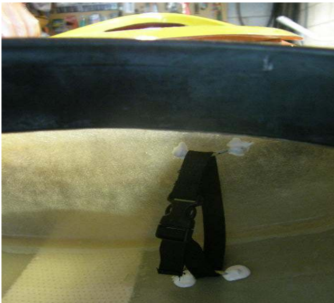
strap for battery box inside day hatch
